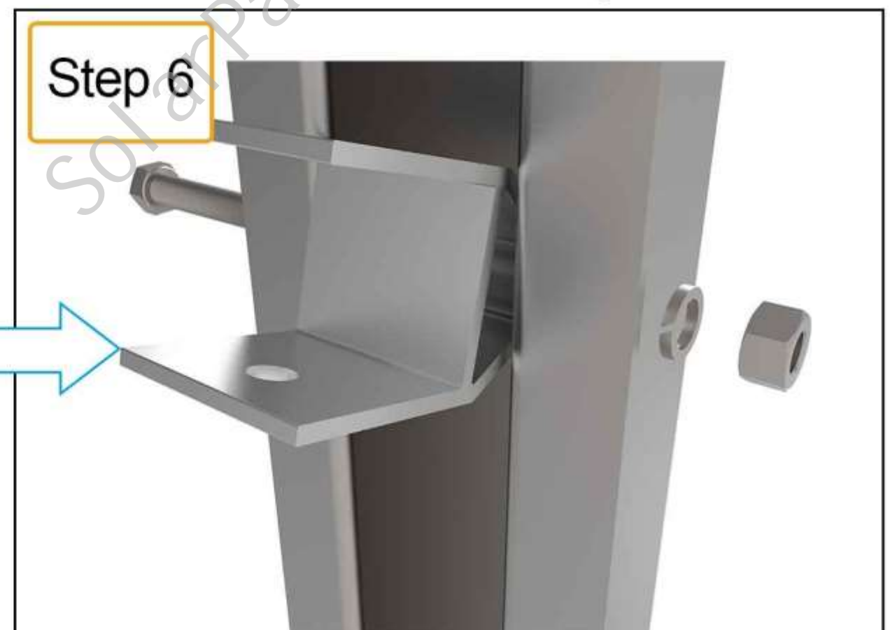
6. Fix the front diagonal brace joint on the column with bolts
