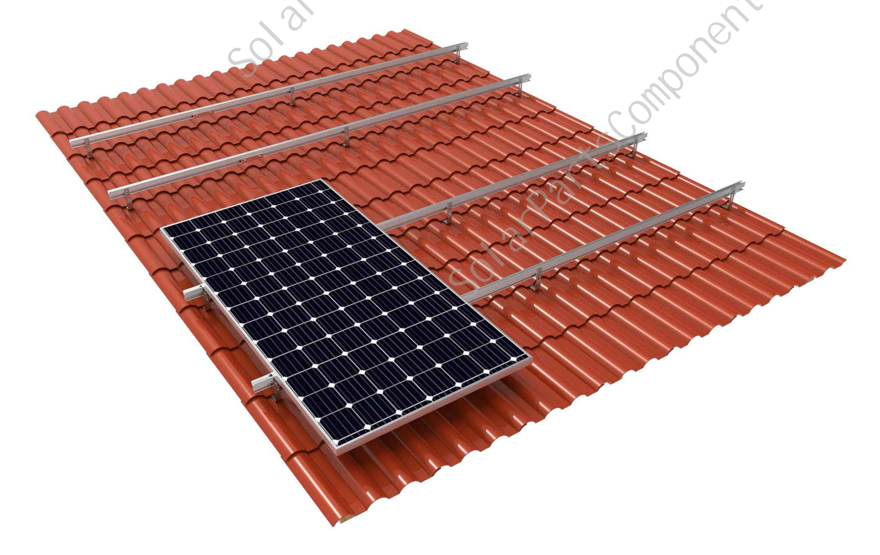
Step six, use the end clamp to lock the side of panels, screw the sliding nut on the end clamp to the bottom of the bolt, and then put it sideways into the groove of the rail.
