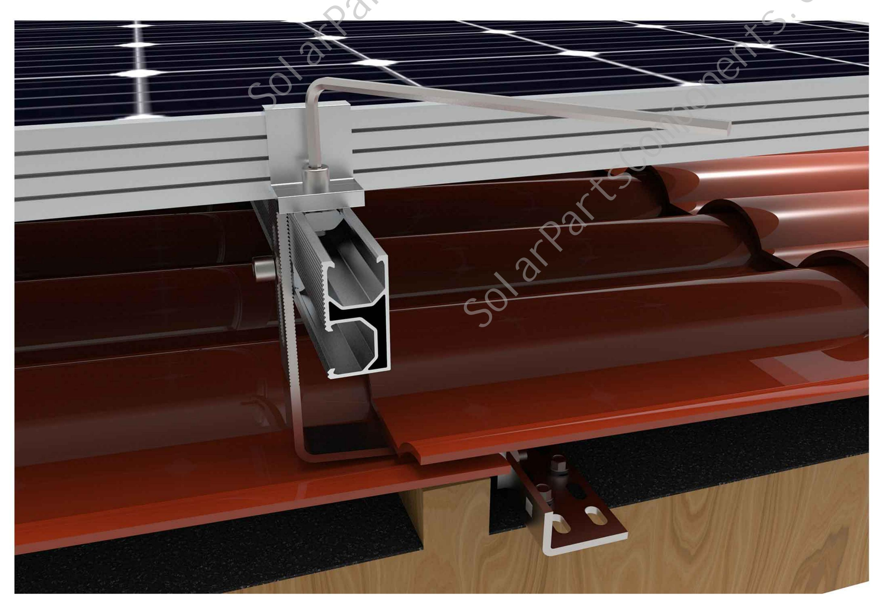
Step seven, The installation of the mid clamp is the same as that of the end clamp. First, screw the sliding nut on the mid clamp to the bottom of the bolt, and then put it sideways into the groove of the rail.
