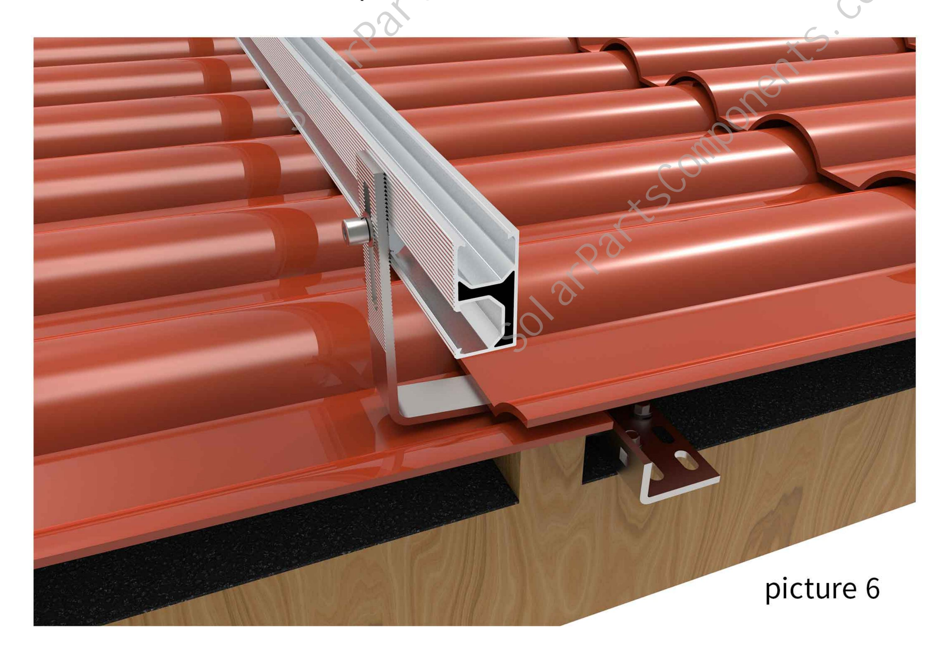
Step four, use the rail splice for the connection between the rail and the rail, insert the connector into the groove on the inner side of the rail, insert 75mm on each side, and then lock the bolts.
