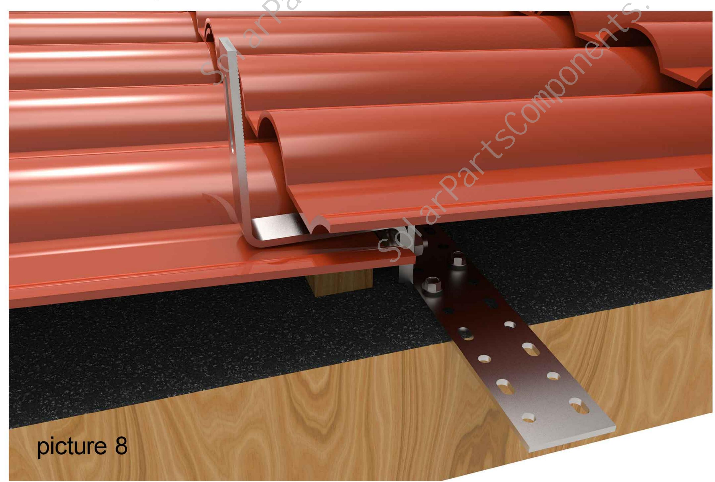
Step seven, install the rail on the stainless-steel hook # 06 with M8\*25 bolts. as picture 9 shows
